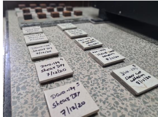
Preparation for Testing Shear Strength
